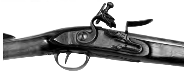
On this French military musket the firing mechanism was called the lock.
